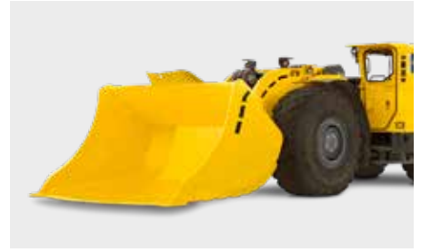
Innovative boom/bucket design and load-sensing hydraulics ensures one-pass mucking while minimizing the fuel consumption.
