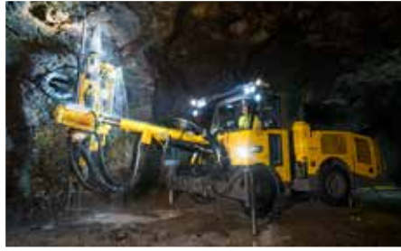
The hydraulic top hammers COP1838+ and MUX+ are made for hard rock drilling in tough conditions.
