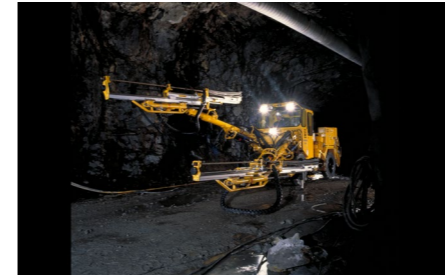
Boomer 282 is world's most popular two-boom face drilling rig with fast, safe and stable drilling performance.
