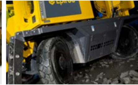
Wheel mounted with high tramming capacity, low diesel consumption, independent front and rear axle steering and four-wheel drive.
